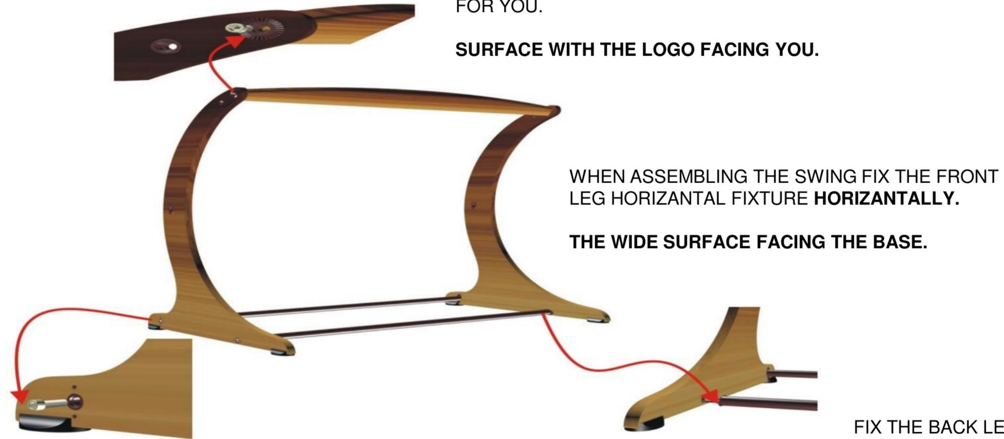
FIX THE BACK LEG HORIZANTAL FIXTURE VERTICALLY.
