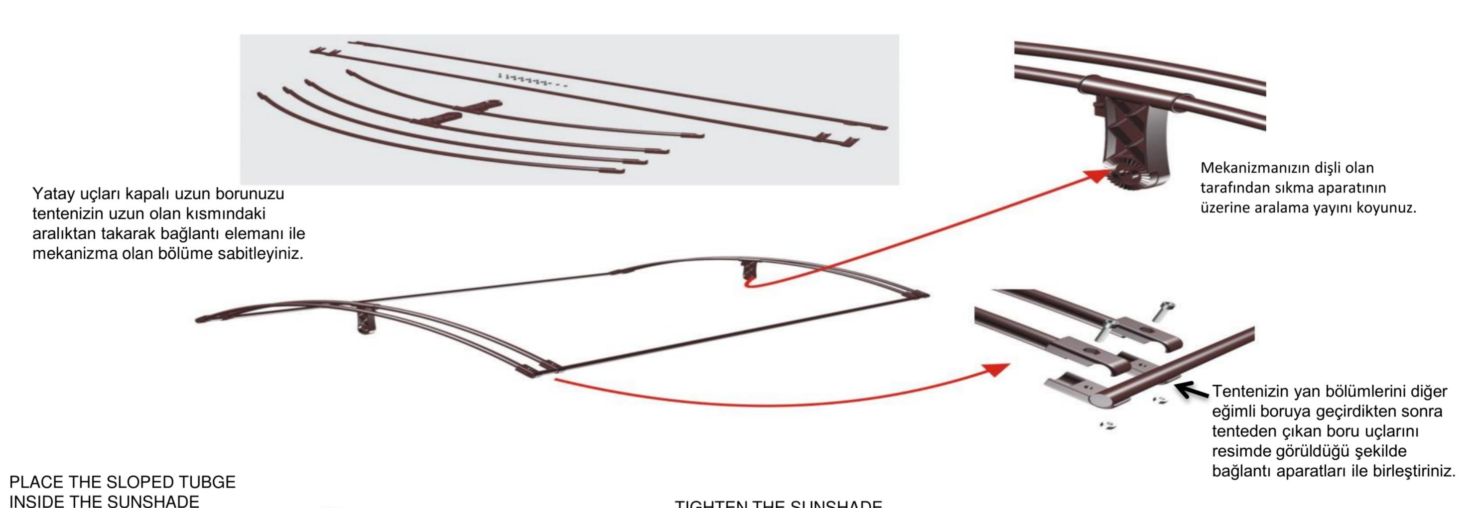
POSITIONING MECHANISM AND FIX THE TIGHTENING APPARATUS ON THE MECHANISM.
